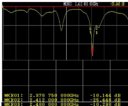
Gambar 8 Hasil Pengujian Return Loss di Network Analyzer
